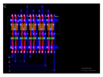
Fig.5. Fully automatic layout design of half subtractor
