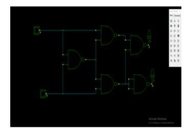
Fig.3. Schematic diagram of half subtractor
