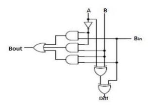
Fig.2. Conventional circuit of full subtractor Table2: truth table of full subtractor
