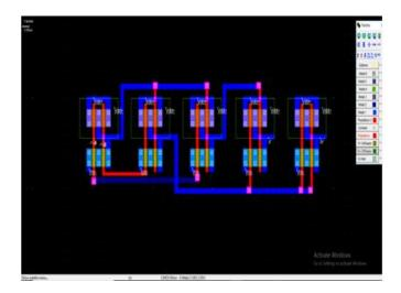
Fig.7. Semi custom layout of the half subtractor
